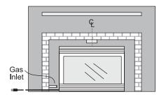
pass through the chimney above the appliance. Move the appliance into the exact location where it is to be installed. Ensure that the Insert is level.
